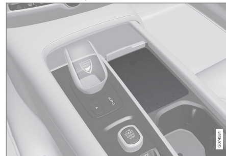
Wireless phone charger in the tunnel console.
