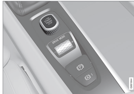
Start knob in the tunnel console.
