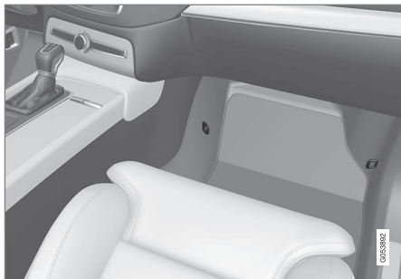
Mounting point locations in the front seat.
