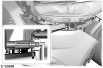
10. Carefully pull the headlamp assembly outward to disengage it from the lower fixing point.
