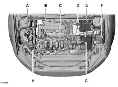
A. Engine coolant reservoir cap
