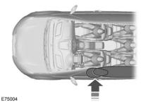
Side curtain airbags located above the trim panels over the front and rear side windows identified by a label or wording on the headliner or roof-pillar trim.
