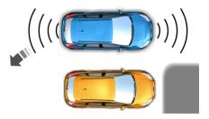
When automatic steering is finished, the touch screen displays a message and a tone sounds, indicating that the active park assist process is done. The driver is responsible for checking the parking job and making any necessary corrections before putting the transmission in Park (P).
