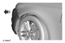
8. Separate the front bumper cover from the fender and pull the fender outward 1.2 inches (3 centimeters).
