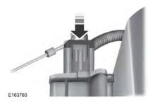
Reconnect the mass air flow sensor electrical connector to the outlet tube. Make sure the locking tab on the connector is in the "locked" position (connector shown from below for clarity).
