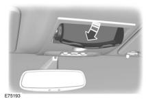
Press near the rear edge of the door to open it.
