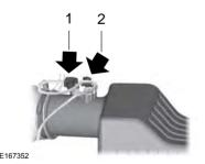
Locate the sensor electrical connector on the air outlet tube (1). This connector will need to be unplugged.
