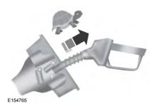
4. After you are done pumping fuel, slowly remove the fuel filler nozzle—allow about 5 to 10 seconds after pumping fuel before removing the fuel filler nozzle. This allows residual fuel to drain back into the fuel tank and not spill onto the vehicle.
