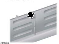
5. Make sure to insert the latch rod into the tailgate hole. Make sure to engage both sides of the locking pins into their holes in the pick-up box.
