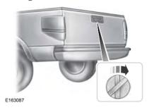
Insert the ignition key into the tailgate lock. Turn it to the right to lock the tailgate. Turn it to the left to unlock the tailgate.
