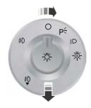
The headlamp control also operates the fog lamps. The fog lamps can be turned on only when the headlamp control is in the parking lamp (second) position, headlamps on (third) position, or autolamp (fourth) position, and the high beams are not turned on.
