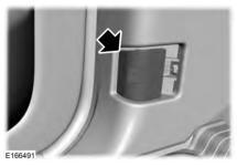
Inside the vehicle, pull the hood release handle located under the left hand side of the instrument panel.
