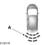
Α Coverage area of up to 6 feet (1.8 meters) from the rear bumper. There is decreased. coverage area at the outer corners of the bumper.
