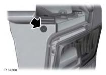
2. Remove the pushpin that holds the air deflector or protective cover to the upper inboard corner of the lamp.
