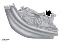
Locate the vertical adjuster on each headlamp. Use a #2 Phillips screwdriver to turn the adjuster either counterclockwise or clockwise in order to adjust the vertical aim of the headlamp.
