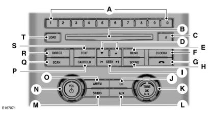
A **Memory presets:** Store your favorite stations for later access. When tuned to any station, press and hold a preset button until sound returns and **PRESET # SAVED** appears in the display. You can also save presets automatically by using the autoset feature:
