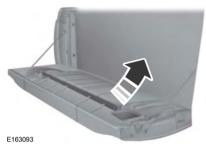
3. Raise the handle upright until you feel it latch and see the lever in the lock position. You only need to use the lever when releasing the grab handle.
