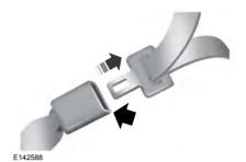
To unfasten, press the release button and remove the tongue from the buckle.
