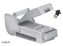
Lift the latch to open the lid and gain access to the optional storage compartment under the center seat cushion.
