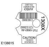
**Note:** Your vehicle's keys came with a security label that provides important vehicle key cut information. Keep the label in a safe place for future reference.
