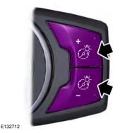
Press repeatedly or press and hold until the desired level is reached.
