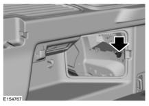
4. Pull the manual override mechanism.
