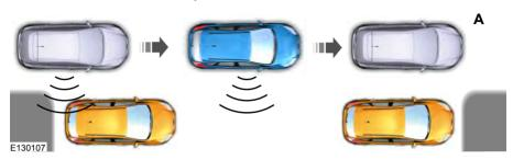
When a suitable space is found, the touch screen displays a message and a chime sounds. Slow down and stop at approximately position (A), then follow the instructions on the touch screen.
