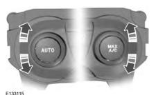
You can set the temperature between  $60^{\circ}F$  (15.5°C) and  $85^{\circ}F$  (29.5°C) in steps of  $1^{\circ}F$  (0.5°C). In position **LO**, 59°F (15°C), the system switches to permanent cooling. In position **HI**,  $86^{\circ}F$  (30°C), the system switches to permanent heating.
