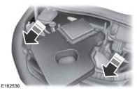
Lift the air cleaner assembly (A) from the mounting studs, then rotate and pull it towards the front of the vehicle.
