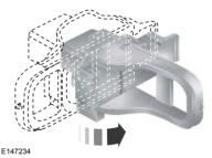
Slide the handle on the service disconnect outboard to the right. For Energi vehicles, slide the handle outboard and to the left.
