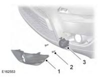
**Note:** You cannot separate the fog lamp bulb from the bulb holder.
