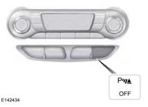
Press the button to switch the system off. It will remain off for the entire ignition cycle. The system can also be switched off through the information display.
