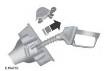
4. Once pumping is complete, slowly remove the fuel filler nozzle. Allow approximately five to ten seconds after pumping fuel before removing the fuel filler nozzle. This allows residual fuel to drain back into the fuel tank and not spill onto the vehicle.
