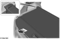
Insert the ends of the cargo shade into the mounting features located behind the rear seat on the rear trim panels to install the cargo shade.
