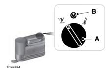
7. Push and turn dial (A) counterclockwise to the sealant position. Turn on the kit by pressing the on and off button (B).
