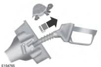
After pumping fuel, slowly remove the fuel filler nozzle. Allow approximately five to ten seconds after pumping fuel before removing the fuel filler nozzle. This allows residual fuel to drain back into the fuel tank and not spill onto the vehicle.
