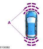
A Coverage area of up to 27 inches (70 centimeters) from the front of the vehicle and about 14 inches (35 centimeters) to the side of the front end of the vehicle. Refer to the reverse sensing section for details on coverage area.
