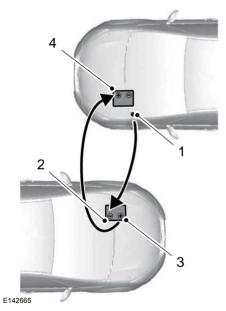
I. Remove the negative (-) jumper cable from the disabled vehicle.
