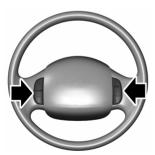
The cruise controls are on the steering wheel. See **Using Cruise Control** (page 43).
