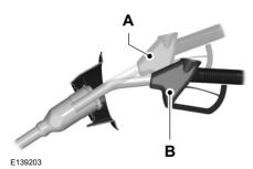
4. Hold the fuel pump nozzle in the lower position B when refueling. Holding the fuel pump nozzle in the higher position A may affect the flow of fuel and shut off the fuel pump nozzle before the fuel tank is full.
