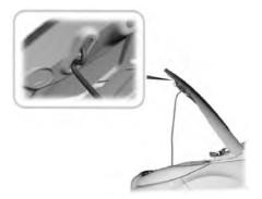
4. Open the hood. Support the hood with the strut.
