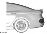
The system uses radar sensors that are located behind the bumper fascia on each side of your vehicle. Any dirt, mud and snow in front of the sensors and/or driving in heavy rain can cause system degradation. Also, other types of obstructions in front of the sensor can cause system degradation. This is referred to as a 'blocked' condition.
