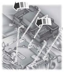
1. Release the two latches, located on both sides of the fuse box.
