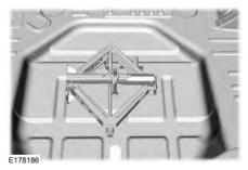
7. Remove the lug wrench and lack from the spare tire compartment.
