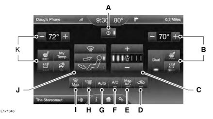
A **Power:** Touch the button to switch the system on and off. Switching off the climate control system prevents outside air from entering the vehicle.
