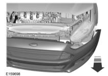
From the front of the vehicle, gently pull the front bumper cover forward 4 inches (10 centimeters) by grasping it next to the headlamp to be serviced and in the lower front of the wheel opening.
