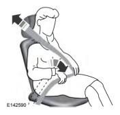
Pregnant women should always wear their safety belt. The lap belt portion of a combination lap and shoulder belt should be positioned low across the hips below the belly and worn as tight as comfort will allow. The shoulder belt should be positioned to cross the middle of the shoulder and the center of the chest.
