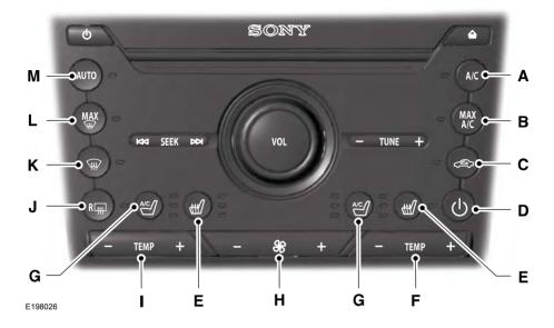
A **A/C:** Press to switch the air conditioning on or off. Air conditioning cools your vehicle using outside air. To improve the time to reach a comfortable temperature in hot weather, drive with the windows open until you feel cold air through the air vents.
