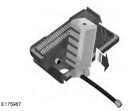
Rotate the sealant canister up 90 degrees and pull away from casing/housing to remove.
