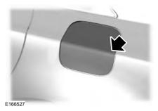
2. Press the center-rear edge of the fuel filler door and release to open.
