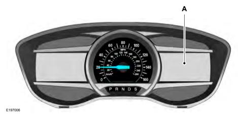
The display is located on the right side of your instrument cluster (A). You can use your steering wheel controls to view and make minor adjustments to active modes without taking your hands off the wheel. For example:
