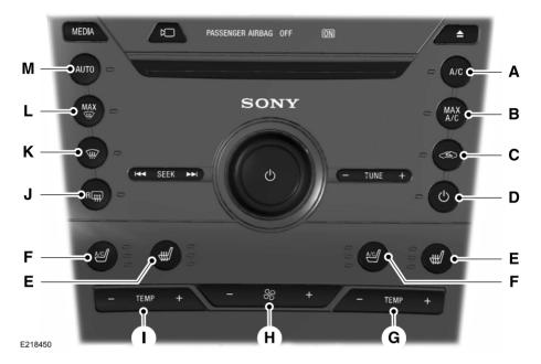
A **A/C:** Press to switch the air conditioning on or off. Air conditioning cools your vehicle using outside air. To improve the time to reach a comfortable temperature in hot weather, drive with the windows open until you feel cold air through the air vents.
