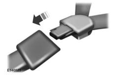
Insert the belt tongue into the proper buckle (the buckle closest to the direction the tongue is coming from) for that seating position until you hear a snap and feel the latch engage. Make sure the tongue is latched securely by pulling on it.
