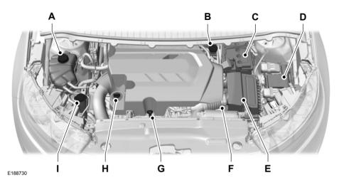
A Engine coolant reservoir. See **Engine Coolant Check** (page 268).
