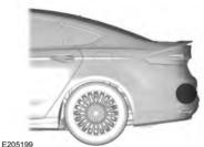
The system uses radar sensors that are located behind the bumper fascia on each side of your vehicle. Do not allow mud, snow or bumper stickers to obstruct these areas, this can cause degraded system performance. See **Blind Spot Information System** (page 209). If the Blind Spot Information System is blocked, Cross Traffic Alert is also blocked. A corresponding message appears in the information display as soon as you shift the transmission into reverse (R).
