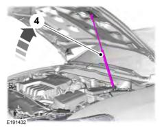
4. Open the hood. The hood strut automatically supports the hood.
