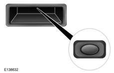
Press the button located in the top of the liftgate pull cup handle to unlatch the liftgate, and then pull on the outside
