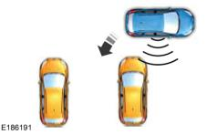
When you shift the transmission into reverse (R), with your hands off the wheel (and nothing obstructing its movement), your vehicle steers itself into the space. The system displays instructions to move your vehicle back and forth in the space.
