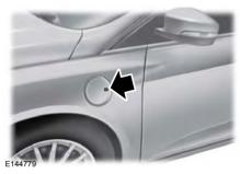
**Note:** Do not force the charge port door open or closed. Forcing the door open or closed damages the charge port.
