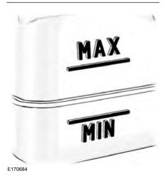
To avoid fluid contamination, the reservoir cap must remain in place and fully tight, unless you are adding fluid.
