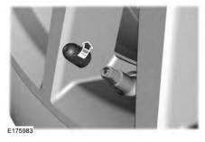
Remove the valve cap from the tire valve.
