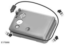
5. Wrap the power cord around the housing and stow the accessory power plug into its storage area.
