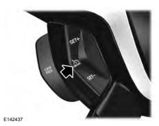
The cruise controls are on the steering wheel.
