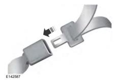
Insert the belt tongue into the proper buckle (the buckle closest to the direction the tongue is coming from) until you hear a snap and feel it latch. Make sure the tongue is securely fastened in the buckle.
