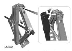
8. To remove the wrench from the jack, turn the hex nut on the jack counterclockwise. This will lower the jack and loosen the mechanical lock.
