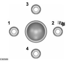
Remove the jack and fully tighten the lug nuts in the order shown. See Technical Specifications (page 233).
