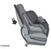
Pull down on the shoulder belt and then grasp the shoulder belt and lap belt together.
