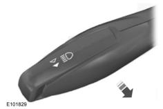
Pull the lever fully toward you to switch the high beams on.
