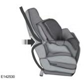
While holding the shoulder and lap belt portions together, route the tongue through the child seat according to the child seat manufacturer's instructions. Be sure the belt webbing is not twisted.
