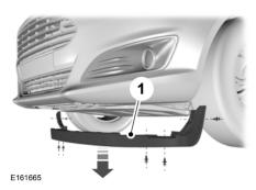
1. Remove the retaining clips to gain access to the lamp assembly.
