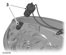
3. Remove the bulb and bulb holder. Remove the bulb.
