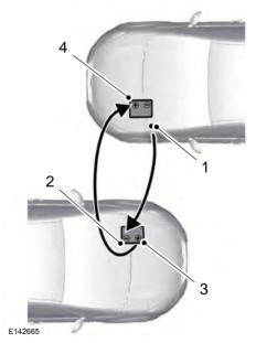
Remove the negative (-) jumper cable from the disabled vehicle.
