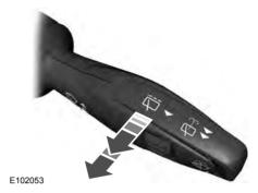
Pull the lever toward you to operate the washers. They will operate for a maximum of 10 seconds. When you release the lever, the wiper will operate for a short time.
