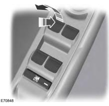
Press the control to open the window.
