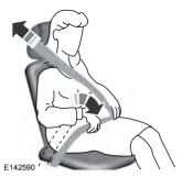
Pregnant women should always wear their safety belt. The lap belt portion of a combination lap and shoulder belt should be positioned low across the hips below the belly and worn as tight as comfort will allow. The shoulder belt should be positioned to cross the middle of the shoulder and the center of the chest.
