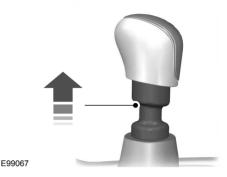
If reverse gear is not fully engaged, press the clutch pedal down and shift the gearshift lever to the neutral position. Release the clutch pedal for a moment, then raise the collar and shift the gearshift lever to reverse again.
