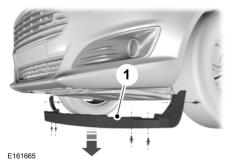
Remove the retaining clips to gain access to the lamp assembly.
