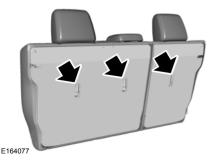
2. Locate the correct anchor on the back panel of the rear seat for the selected seating position.
