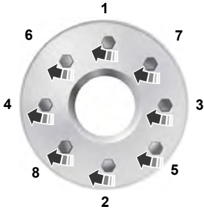
8-lug nut torque sequence
